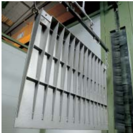
Sand-blasting access ramps
